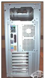
These two screws plus those in the back hold attach the side panel to the case with no tabs or slots being employed, the only other cases I've seen, that has used this method is the expensive Enermax Aluminum cases. Of course, this means that every panel of the outer shell must be perfectly cut and fitted No fear, the Meridian M-2015 aluminum case has been assembled with the precision you would expect in much more costly cases!
