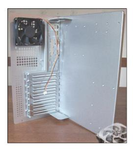
Meridians slide-out removable motherboard tray is one of the all time best that I've worked on, only Cooler Master's may be better and that's debatable. Like every other part of the M-2015 the motherboard tray perfectly aligns to the rest of the case and even when fully loaded, does not bend or warp.
